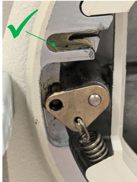
Figur 2: Acceptable lubrication on/near the bronze link
